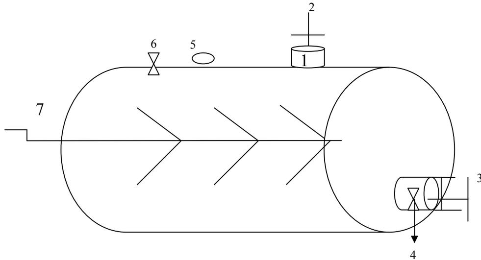
**Figure 11** Schematic diagram of 1.5m<sup>3</sup> digester with stirrer:- 1- Inlet open, 2- screw closer, 3- outlet open with screw closer, 4- sample getting out valve (0.75inch), 5- pressure gauge, 6- gas valve (0.5 inch), 7- manual stirrer. Each inlet or outlet opening is of 8 inch diameter.
