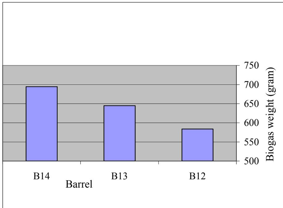
Results of samples (B12, B13, B14, B15, B16, B17, and B18) – figure 19 - indicate that sample of equal ratios (B18) from the three animal dung types (cow, sheep and goat, chicken) produces the largest quantity of biogas (63.1 g/kg waste) with reaching its maximum production at shorter time. The reason is not so clear, it may be returned to the reaching best total solids ratio or best C/N ratio among different waste types.
