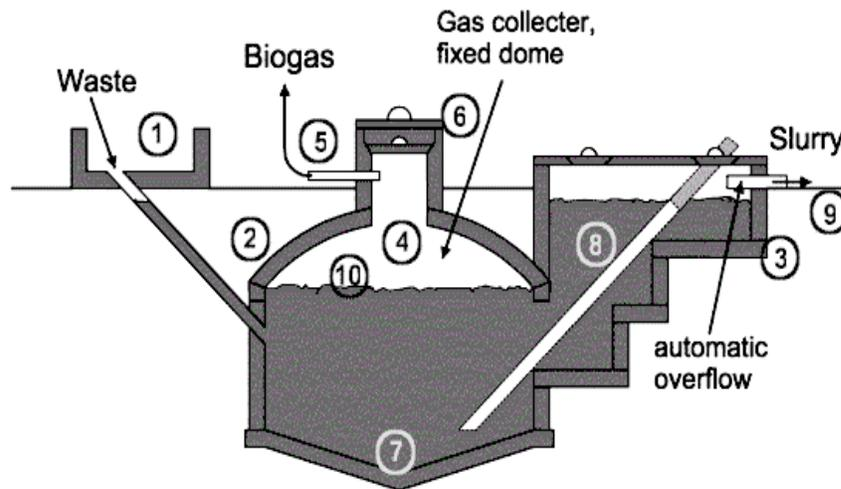
**Figure 7** Fixed dome plant Nicarao design: 1. Mixing tank with inlet pipe and sand trap. 2-Digester. 3. Compensation and removal tank. 4. Gasholder. 5. Gas pipe, 6-Entry hatch, with gastight seal. 7. Accumulation of thick sludge. 8. Outlet pipe. 9. Reference level. 10. Supernatant scum, broken up by varying level
