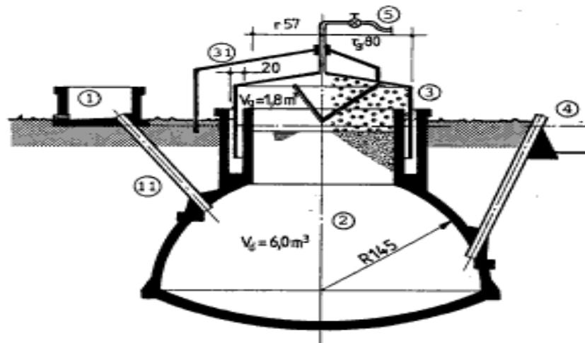
**Figure 8** Water-jacket plant with external guide frame. 1- Mixing pit, 11- Fill pipe, 2- Digester, 3-Gasholder, 31- Guide frame, 4- Slurry store, 5- Gas pipe.
