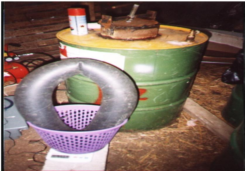
**Photo 11** Weighting biogas by digital balance.
