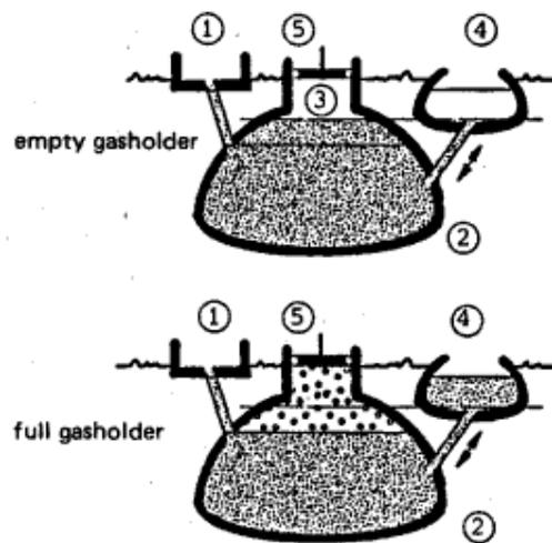
**Figure 4** Basic function of a fixed-dome biogas plant, 1- Mixing pit, 2- Digester, 3- Gasholder, 4- Displacement pit, 5- Gas pipe
