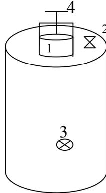
**Figure 10** Schematic diagram of a barrel digester:- 1- inlet opening (8 inch diameter), 2- gas valve (0.5 inch), 3- valve to get out slurry samples (0.5 inch), 4- screw to close tightly inlet cover.
